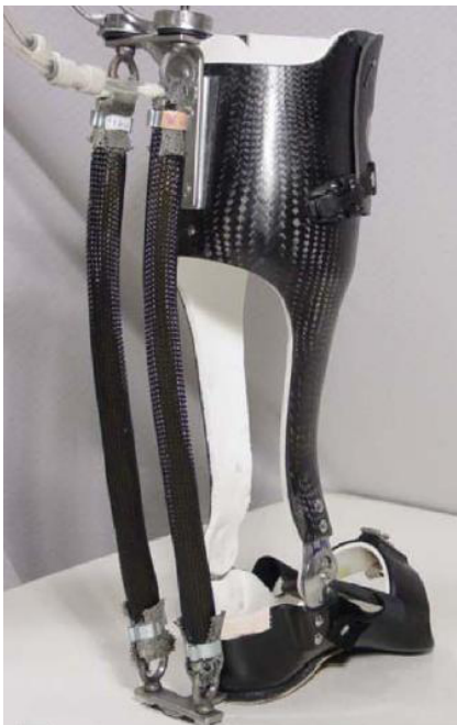
◀ Slika 5 Ortoza za stopalo pokretana pneumatskim mišićima (prema: K.E. Gordon, G.S. Sawicki, D.P. Ferris: Mechanical performance of artificial pneumatic muscles to power an ankle-foot orthosis , Journal of Biomechanics)
