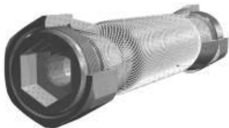
▲ Slika 8 Neke izvedbe umjetnih pneumatskih mišića. (prema: F. Daerden, D. Lefeber: Pneumatic Artificial Muscles: actuators for robotics and automation, European Journal of Mechanical and Environmental Engineering 47; 2002.)
