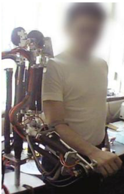
▲ Slika 4 Mehanički sustav za pokretanje ljudske ruke (prema: N.G. Tsagarakis, D.G. Caldwell: Development of a 'Soft-Actuated' Exoskeleton for Use in Physiotherapy and Training, Autonomous Robots 15; 2003.)
